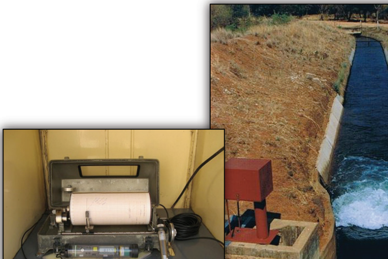
Figure 5: Flow data collected via chart recorders and electronic loggers to be incorporated in the WAS
